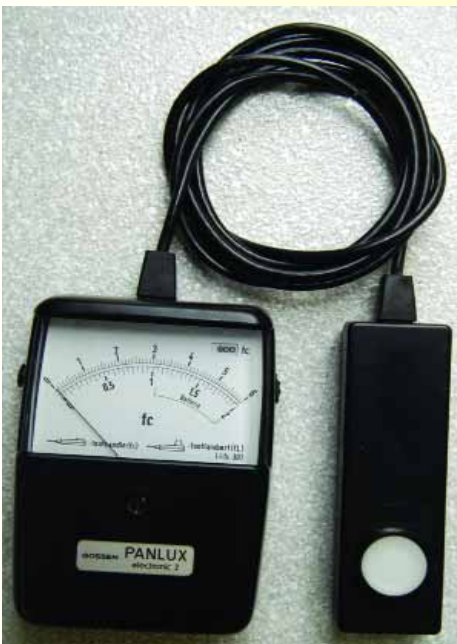
Although this simple light meter measures light in foot-candles rather than PAR, it still gives an accurate idea of light distribution.
